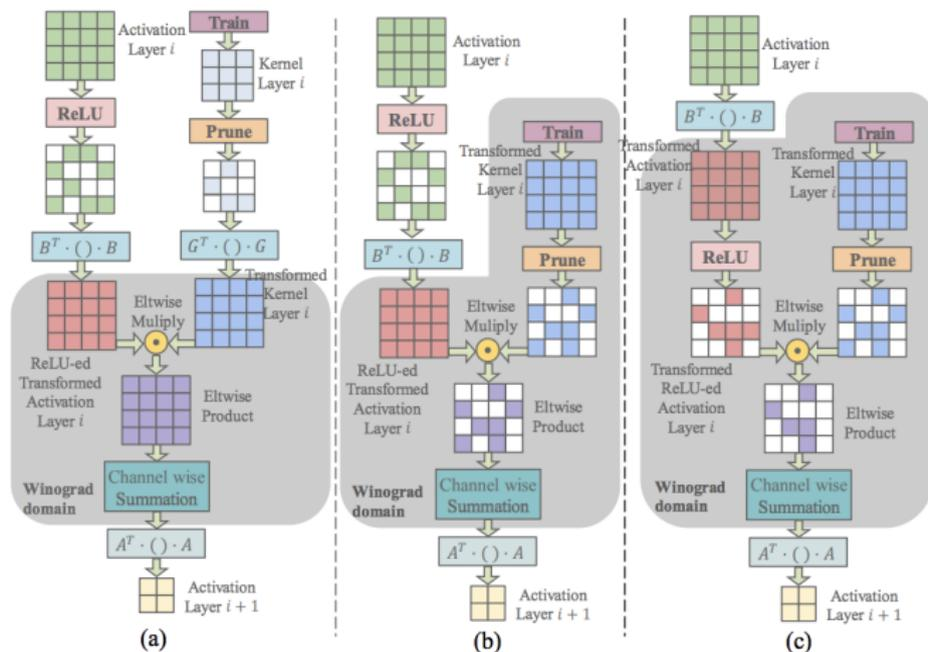
Figure 1: Combining Winograd convolution with sparse weights and activations. (a) Conventional Winograd-based convolution fills in the zeros in both the weights and activations. (b) Pruning the  $4 \times 4$  transformed kernel restores sparsity to the weights. (c) Our proposed Winograd-ReLU CNN. Moving the ReLU layer after Winograd transformation also restores sparsity to the activations.
