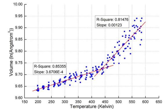
**Figure 8.** The volume-temperature relation of 85% crosslinked BADGE-IPDA resin system
