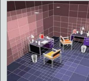
Radiosity problem in computer science, objects in space divided into subsurface to calculate view factor.
