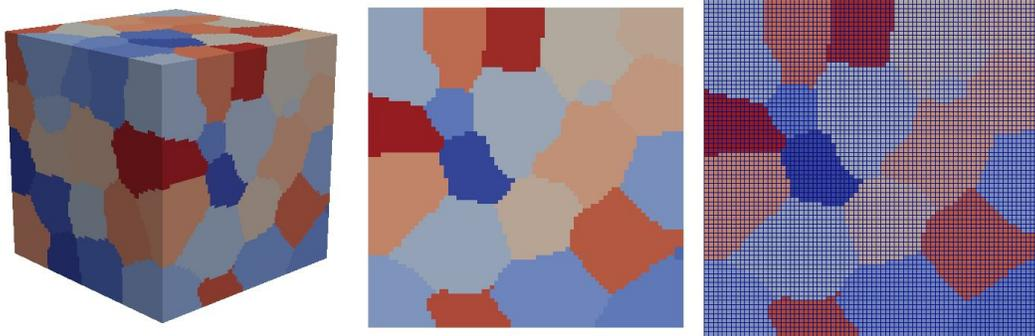
**Figure 4:** Microstructural grains created using Dream3D in the cube example from Figure 2.
