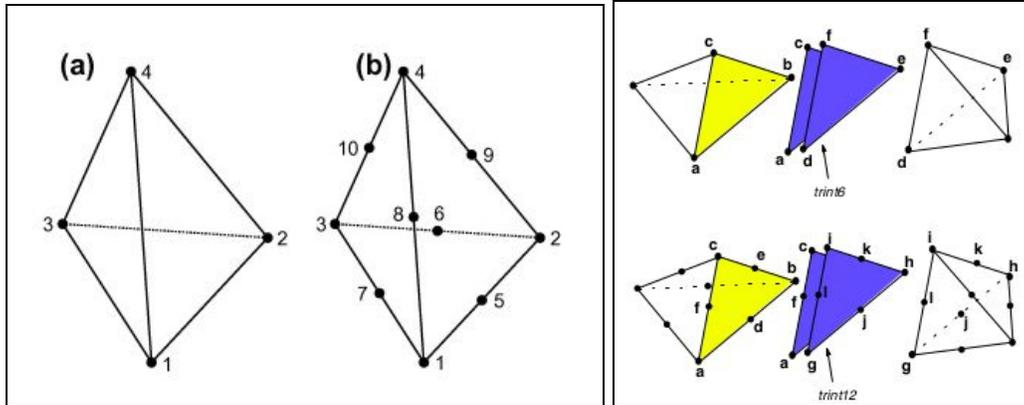
**Figure 6:** (a) Four node tetrahedral (b) Ten node tetrahedral interfaces **Figure 7:** Six node and twelve node interfaces
