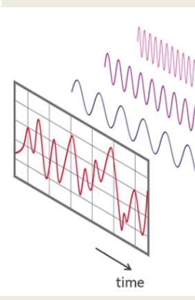
The FFT reduces the time complexity from O(N<sup>2</sup>) (DFT) to O(NlogN), which is feasible for large data.
